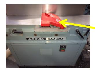
Self-adjusting guard that covers the rotating cutting head must be in place.
