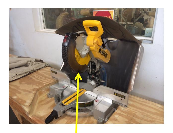
Self-adjusting guard protects the operator from the portion of the blade that is above the table. This guard is to be in place and functioning properly before saw is to be used.
