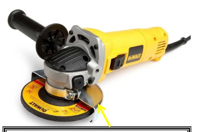
Grinder must have a guard for the grinding disc. The maximum exposure angle allowed is 180° and the guard shall be located so as to be between the operator and the wheel during use.
