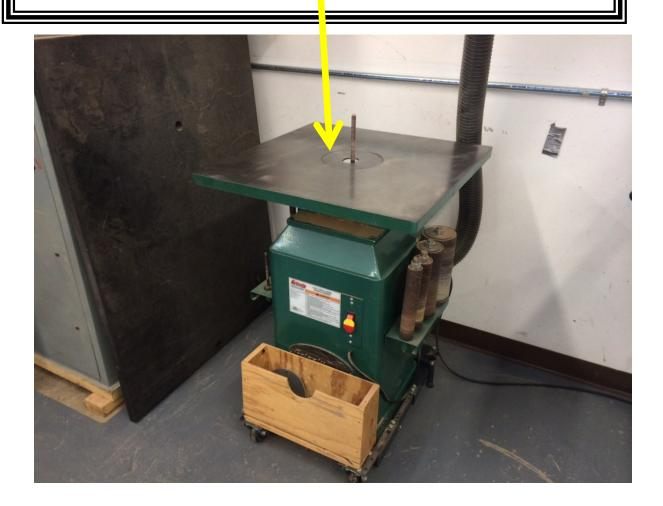
The cover for the power transmission needs to be closed and secure. The removable access panel is on the back of the machine.
