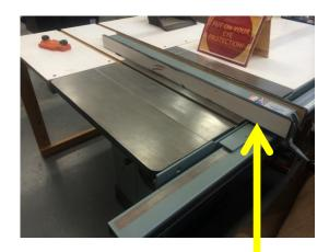
Saw blade should be lowered and under rip fence when not in use.
