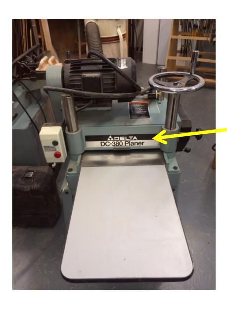
Cutter heads must be completely enclosed, except for the opening needed to feed the stock into the tool.
