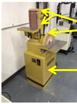
Top and sides of belt to be guarded. Perimeter and back of disc to be guarded.
