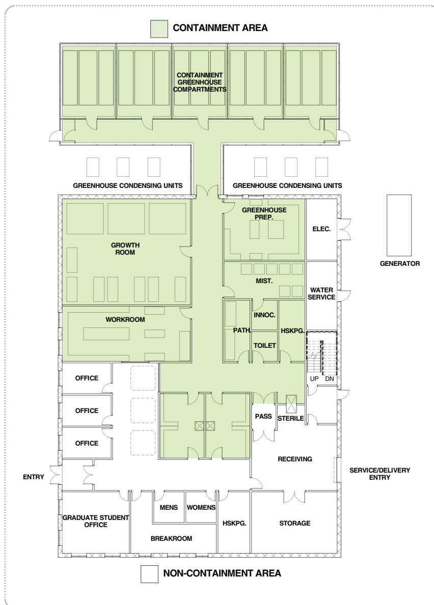
FIGURE 7. Typical Containment Facility Floor Plan*
